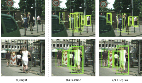
Figure 7. Visualized comparison of predicted bounding boxes before NMS of baseline and RepBox. In the results of RepBox, there are fewer predictions lying in between two adjacent ground-truths, which is desirable in crowd scenes. More examples are shown in supplementary material.
