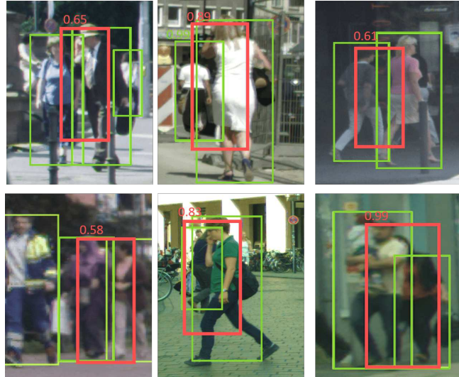
Figure 4. The visualization examples of the crowd errors. Green boxes are correct predicted bounding boxes, while red boxes are false positives caused by crowd occlusion. The confidence scores outputted by detectors are also attached. The errors usually occur when a predict box shifts slightly or dramatically to neighboring ground-truth object (e.g., top-right one), or bounds the union of several overlapping ground-truth objects (e.g., bottom-right one).
