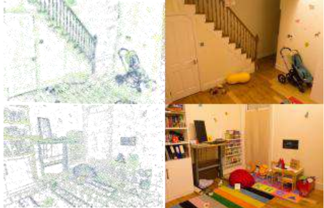
Figure 6. Anchor feature clustering. We cluster anchor features (DB-PLAYROOM) into 3 clusters using K-means [25] and visualize the result. The clustered features show clues of scene contents, e.g. the banister, stroller, desk and monitor can be clearly identified. Anchors on the wall and floor are also respectively grouped together. This shows that our approach improves the interpretability of 3D-GS model, and has the potential to be scaled-up on much larger scenes exploiting reusable features.
