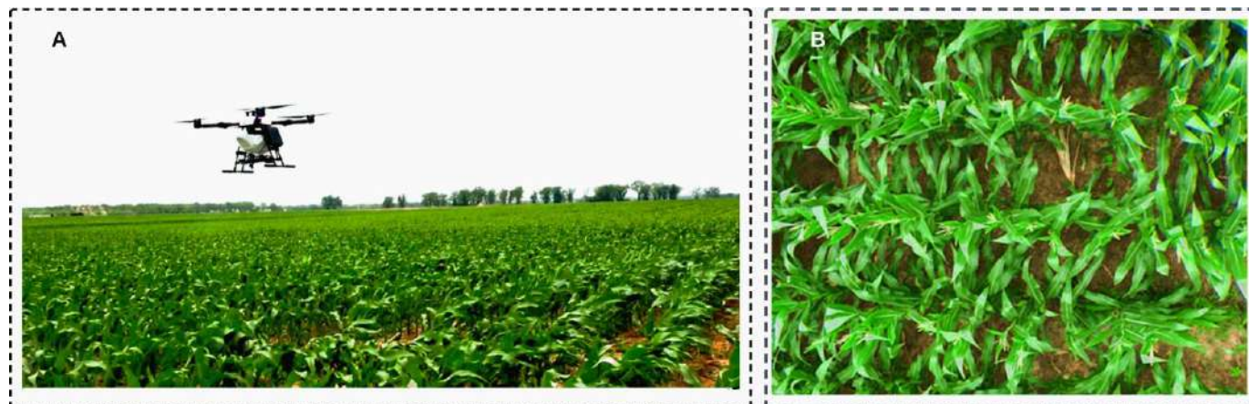
Figure 3. (A) The customized spot-sprayer UAS flying over an experimental corn field (containing some cotton plants planted to mimic as volunteer cotton (VC) plants) capturing five band multispectral images; (B) RGB (Red, Green Blue) composite image showing a section of experimental plot where corn at vegetative tassel state (VT) and some cotton plants mimicking as VC plants can be seen.
