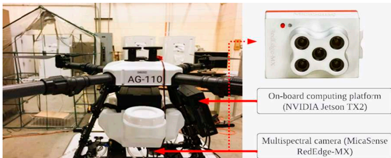
Figure 2. A customized sprayer UAS (broadcast sprayer converted to spot sprayer) with RedEdge-MX multispectral camera for capturing aerial imagery and NVIDIA Jetson TX2 computing platform [7].
