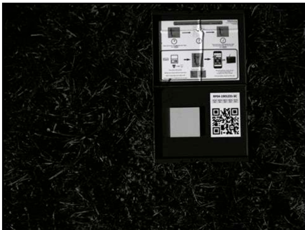
Figure 4. Reflectance panel of type RP 04 image with blue band sensor of RedEdge-MX camera taken on the day of flight.
