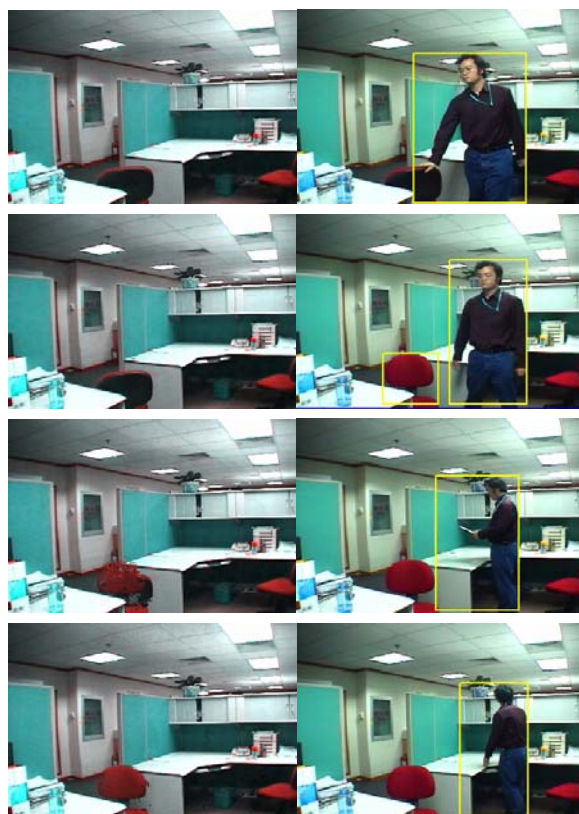
Figure 7. Left object, a person move a red chair into different place. These images are captured at frame #1, frame #13, frame #98, frame #189. The first column contains the background model. The second column contains the bounding box of the detected moving object.
