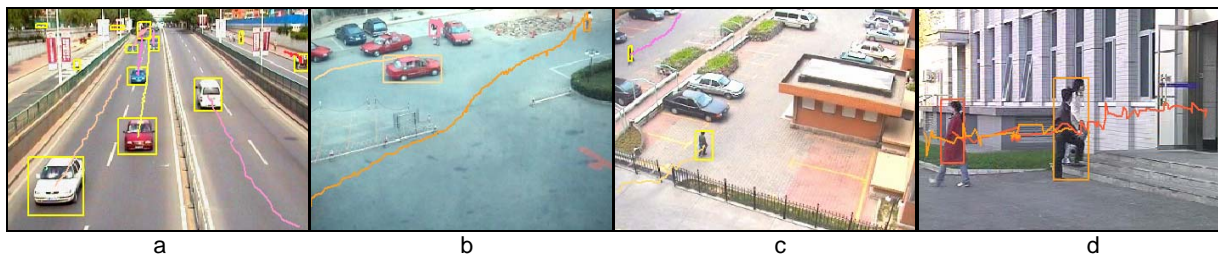
Figure 7. Real time multiple object detection and tracking results in real surveillance scene. These sequences are selected in the real time surveillance system and represent the typical scenes in a residential area. a) Road surveillance. b) Entrance of parking lot. c) Back yard. d) Entrance of the building.
