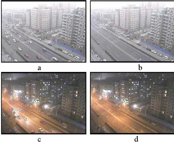
Fig.3 Background estimation. The first column a), c) contains the input video of day and night. The second column b),d) contains the estimated background.
